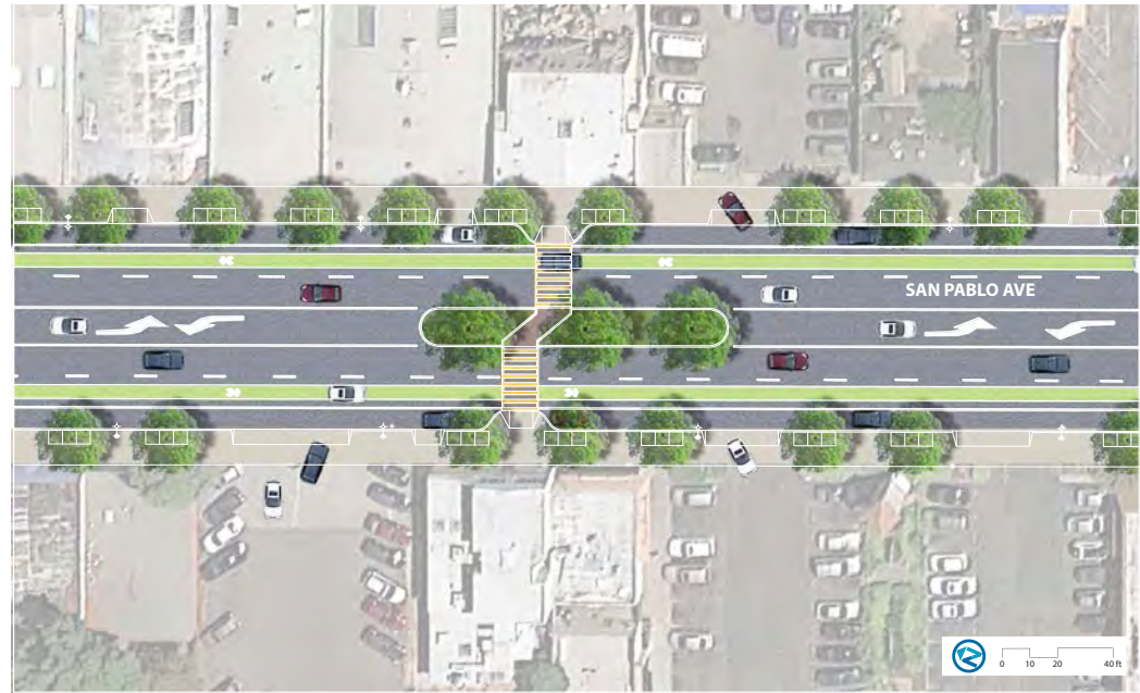
Figure 3-30 Midblock Crossing Between Marin and Monroe - Plan View
