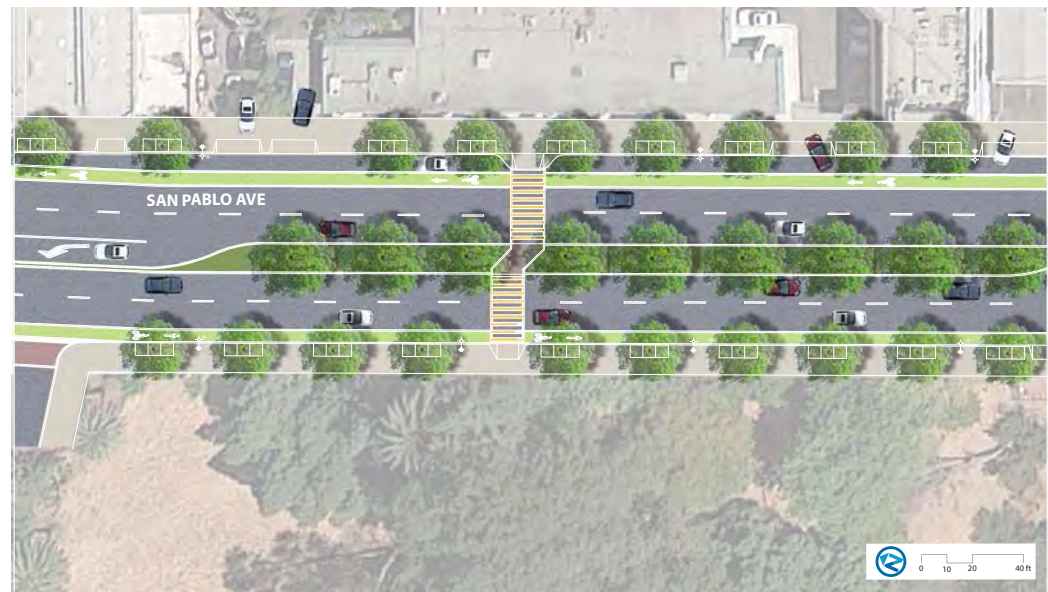
Figure 3-30 Midblock Crossing Between Marin and Monroe - Plan View
