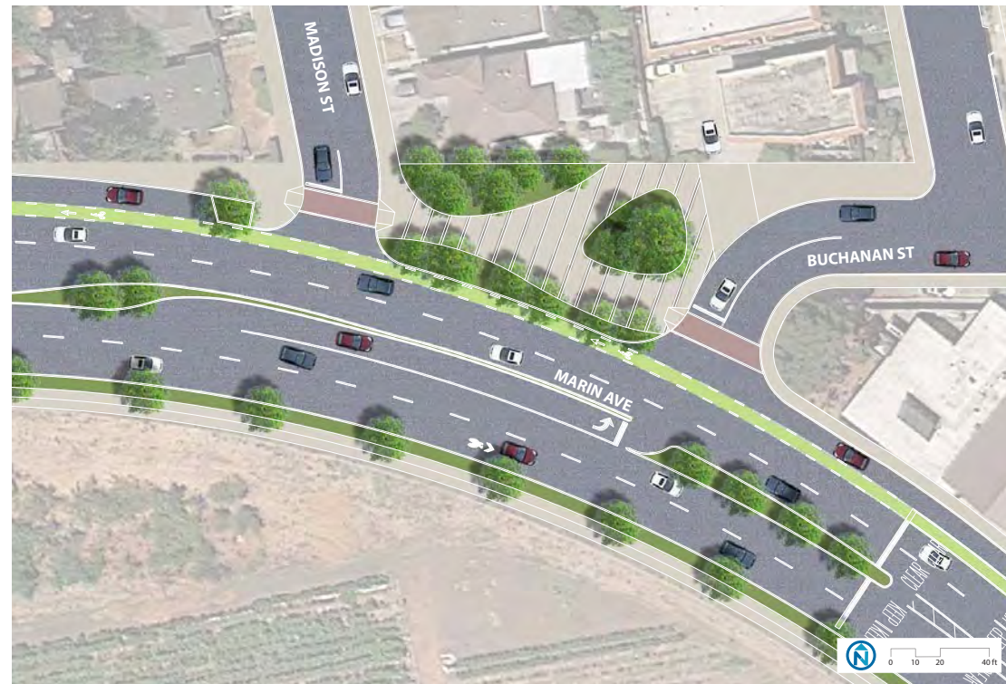
Figure 3-40 Reconfigured Intersection of Marin Avenue and Buchanan Street - Plan
