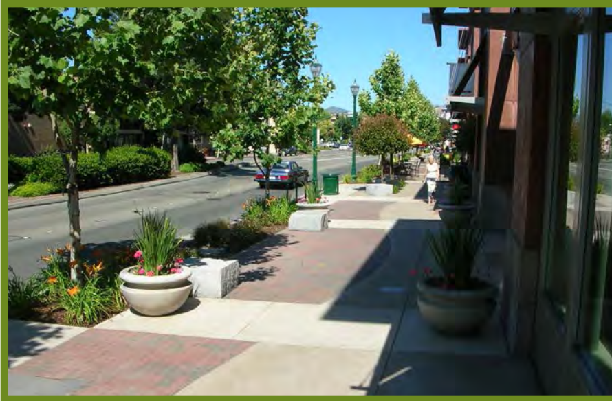
Decorative paving can help define the amenity and pedestrian zones of the sidewalk (Walnut Creek, CA).
