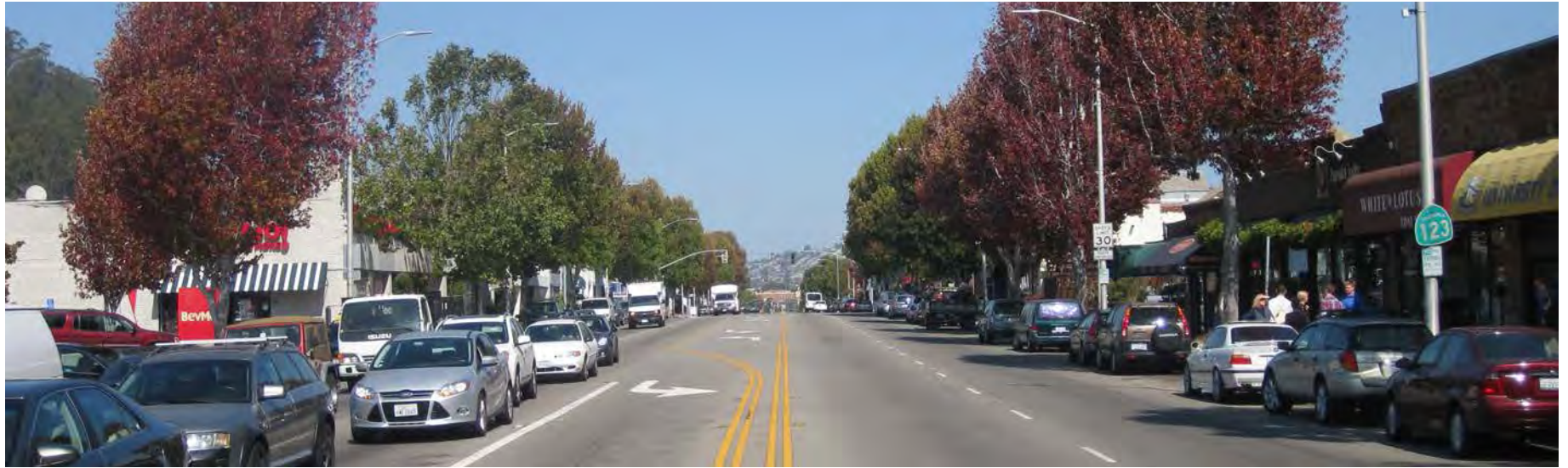
San Pablo is a wide street with broad travel lanes that encourage speed at the expense of pedestrians and locally serving retail establishments. The street is lined with mature, widely spaced trees which do not adequately frame the street and create an inviting sidewalk environment. Retail signs are typically oriented toward the street only and, due to their height, conflict with trees, suggesting that an alternative signage strategy is needed to attract due attention to the retail frontages.
