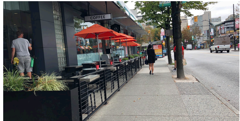
Sidewalk elements such as fences, landscape planters, and fixtures, furnishings, and equipment need to be clear of the pedestrian pathway.
