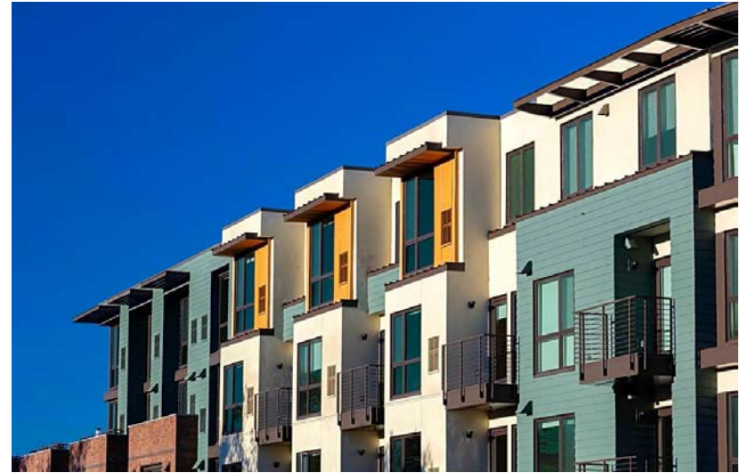
Modulation using recesses, varied setbacks, and roof line changes, help to break up long rectangular facades. The top image is an example of a modulated building facade. The bottom image is an example of roofline variation with changes in height, setback, color, awnings, balconies, and changes in the material to create visual interest.
