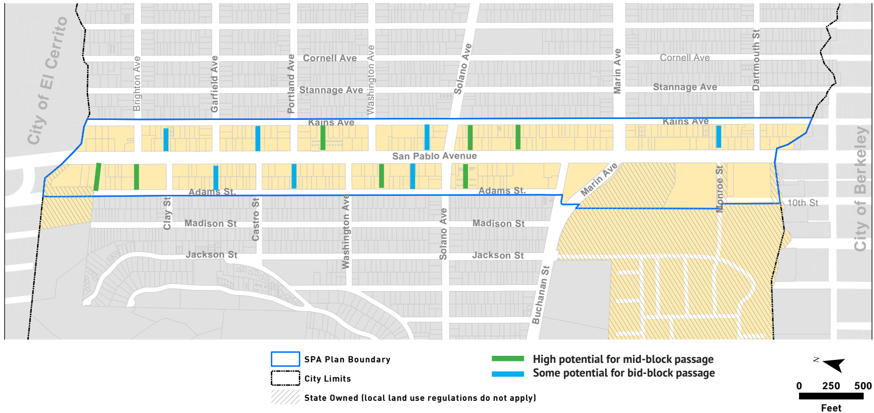
FIGURE 3-2: POTENTIAL LOCATIONS OF MID-BLOCK PASSAGES
