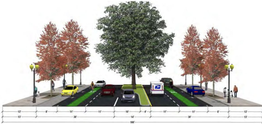
Option 3 Section for shared lane markings from Clay Avenue to Buchanan Street.
